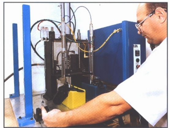
Small bench-top Hot Air fixture for mirror brackets.
