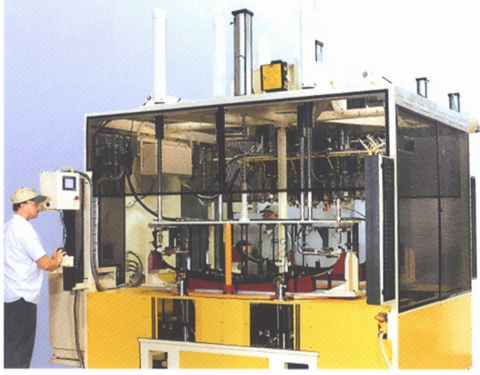
Two-station Hot Air dial machine for automotive grilles. Clip driving also takes place on the two-sided operation machine.
